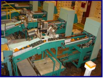
The weigher PGC-2 is prepared to place a label machine with bicones table at the entrance, to label 100% of the fruit to work.
